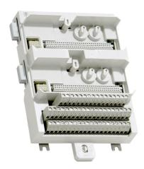
S800 I/O is a comprehensive, distributed, and modular process I/O system that communicates with parent controllers over industry-standard field buses. Module Termination Units (MTUs) host S800 I/O modules and are keyed to ensure the correct module is used. Many Module Termination Units (MTUs) options are available for various S800 I/O modules to meet your project requirements.
